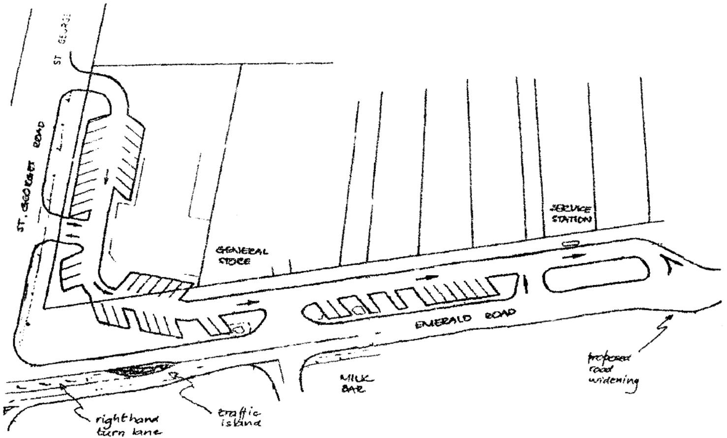
The Shire Engineer's Department has proposed the above scheme to meet the parking requirements outside the General Store. Note the one-way traffic flow and the new entrance in St. Georges Road, as well as additional turning lanes and traffic islands. The plan can be inspected at the General Store. Mr. Warwick Bayley, the shire Engineer, will attend the next Upper Beaconsfield Association meeting on 1st April to discuss the proposal.
